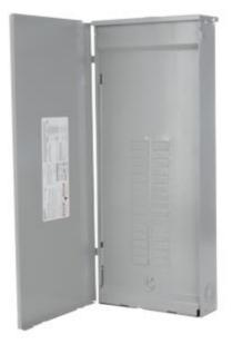
SIEMENS LOW VOLTAGE ES SERIES LOAD CENTER. MAIN LUG WITH 30 1-INCH SPACES ALLOWING MAX 54 CIRCUITS. 3-PHASE 4-WIRE SYSTEM RATED 120/240V OR 120/208V (200A) 100KA INTERRUPT. SPECIAL FEATURES: ALUMINUM BUS, GRAY TRIM, NEMA TYPE3R ENCLOSURE FOR OUTDOOR USE.
