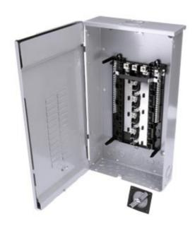
SIEMENS LOW VOLTAGE ES SERIES LOAD CENTER. MAIN LUG WITH 24 1-INCH SPACES ALLOWING MAX 42 CIRCUITS. 3-PHASE 4-WIRE SYSTEM RATED 120/240V OR 120/208V (200A) 100KA INTERRUPT. SPECIAL FEATURES: ALUMINUM BUS, GRAY TRIM, NEMA TYPE3R ENCLOSURE FOR OUTDOOR USE.
