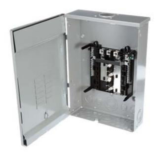
SIEMENS LOW VOLTAGE ES SERIES LOAD CENTER. MAIN LUG WITH 12 1-INCH SPACES ALLOWING MAX 24 CIRCUITS. 3-PHASE 4-WIRE SYSTEM RATED 120/240V OR 120/208V (200A) 100KA INTERRUPT. SPECIAL FEATURES: ALUMINUM BUS, GRAY TRIM, NEMA TYPE3R ENCLOSURE FOR OUTDOOR USE.
