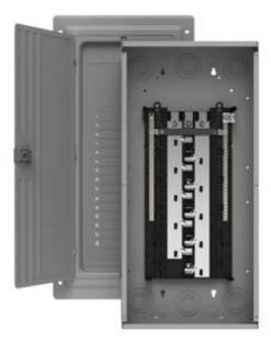
SIEMENS LOW VOLTAGE ES SERIES LOAD CENTER. MAIN LUG WITH 30 1-INCH SPACES ALLOWING MAX 54 CIRCUITS. 3-PHASE 4-WIRE SYSTEM RATED 120/240V OR 120/208V (200A) 100KA INTERRUPT. SPECIAL FEATURES: ALUMINUM BUS, GRAY TRIM, NEMA TYPE1 ENCLOSURE FOR INDOOR USE.
