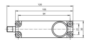
Bore hole and countersinking for screws/hexagon M4
