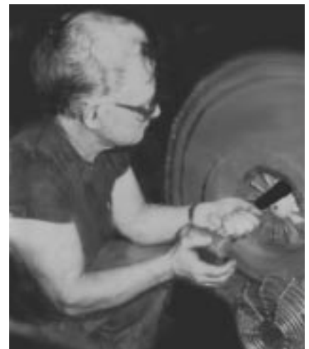
Photo 3: Technique for pushing new impeller onto shaft
