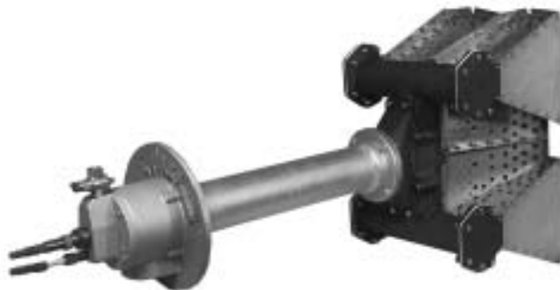
36" back inlet "H" INCINO-PAK® Burner section shown with (4) COMBUSTIFUME® Burner end plates; includes spark ignitor, pilot gas adjustable orifice cock, raw gas pilot, and arranged for mounting of customer's UV scanner
