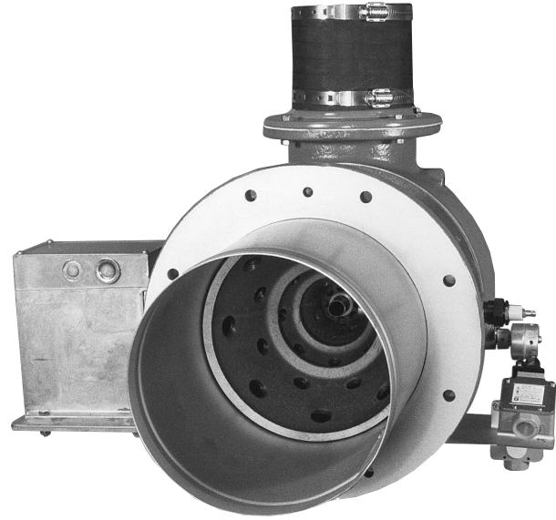
View into metallic cone of Model EB-3 OVENPAK®-II Burner, arranged for external blower source, with connecting base and linkage assembly to adapt customer's automatic control motor, and optional low fire start switch arrangement. Inlet air piping uses flexible connector set.
