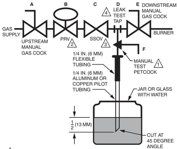
Fig. 16. Valve leak test.
