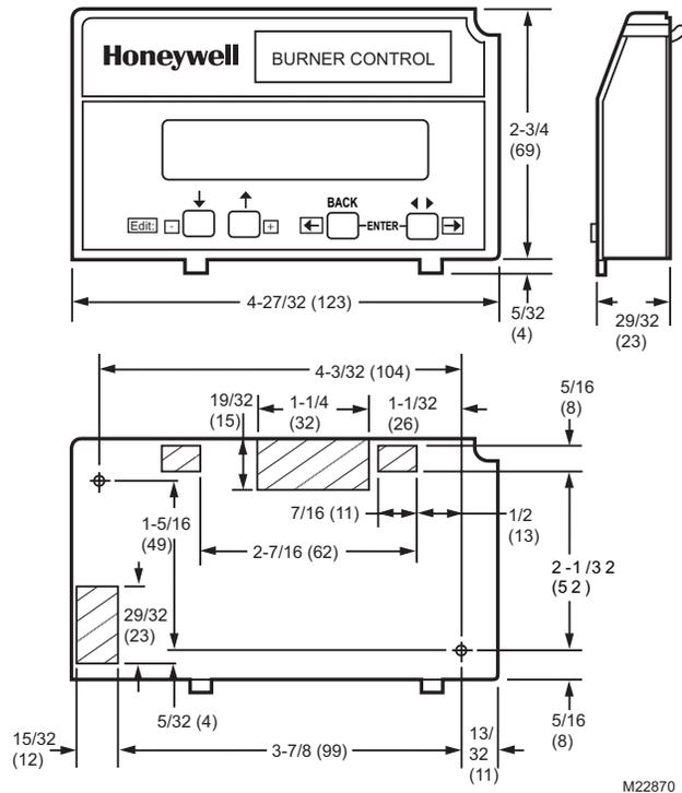
Fig. 1. Approximate dimensions of S7800A1001 in. (mm).
