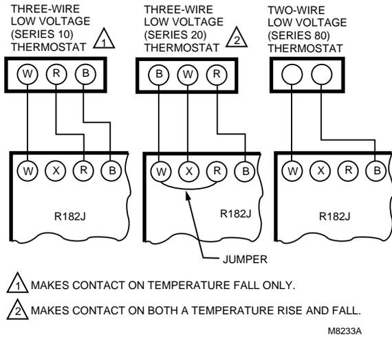
**Fig. 6—Internal schematic and typical hookup for R482J.**
