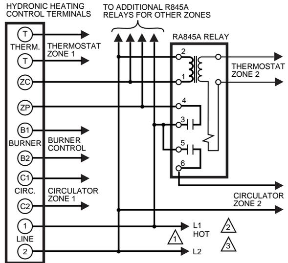
**Fig. 8—R845A hookup for controlling two loads.**
