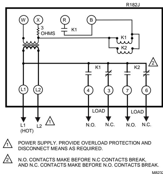
**Fig. 5—Thermostat connections for R182J.**
