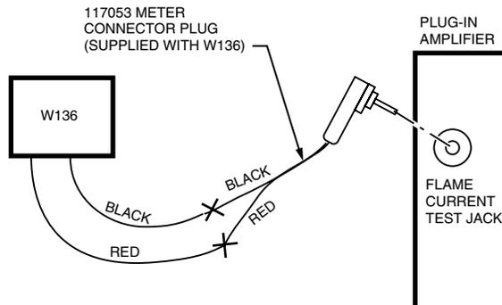
IF 117053 METER CONNECTOR PLUG IS NOT AVAILABLE (R7289A RECTIFICATION AMPLIFIER ONLY)
