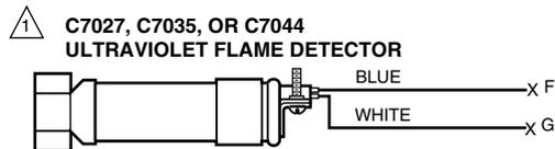
**⚠** C7027, C7035, AND C7044 FLAME DETECTOR LEADS ARE COLOR CODED BLUE AND WHITE. THE BLUE LEAD MUST BE CONNECTED TO THE F TERMINAL AND THE WHITE LEAD MUST BE CONNECTED TO THE G TERMINAL. THIS CIRCUIT IS DC AND THE UV SENSING TUBE IS POLARITY SENSITIVE. REVERSING THE LEADS EVEN MOMENTARILY CAN DAMAGE OR DESTROY THE UV TUBE.
