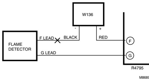
Insert a 117053 Meter Connector Plug, wired color-to-color to the W136 leadwires, into the test jack on the amplifier (Fig. 10). This automatically puts the microammeter in series with the flame detector.
