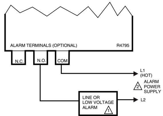
**⚠** IF A LINE VOLTAGE ALARM IS USED, THE R4795 MUST BE MOUNTED IN A SUITABLE ENCLOSURE.
