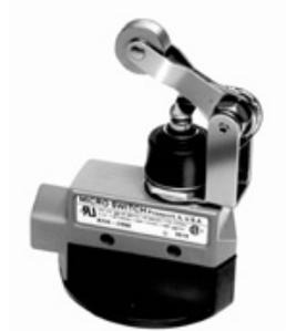
**Enclosed Switches Series V6: Top Roller Arm Actuator, Adjustable with Steel Roller; 1NC 1NO SPDT Snap Action; 0.5 in - 14NPT conduit**
