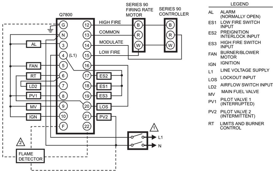
1 120 VAC, 50/60 HZ POWER SUPPLY, RM7850A; 220-240 VAC, 50/60 HZ POWER SUPPLY, EC7850A.
